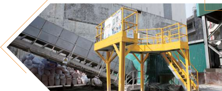
Safe working platforms specifically designed to assist drivers with truck cleaning.
